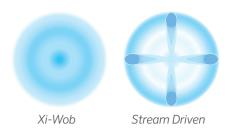
In this example, the Xi-Wob is instantaneously spreading the same amount of water over an area five times greater than the area covered by the spray nozzle.
